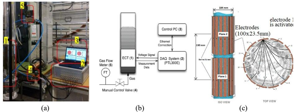
Figure 1. (a) Actual system used for fluidization studies using a fluidizing bed column (FBC) with a dedicated ECT measurement system; (b) Schematic diagram of the FBC with installed twin plane ECT sensor and its data acquisition and storage devices; (c) Geometry of the 12-electrodes twin-plane ECT sensor installed on the FBC as the item 1, and “TOP VIEW” shows as example the capacitance measurement between each pair of electrodes, with electrode no. 1 activated.
