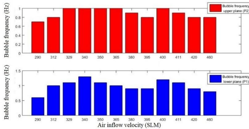
Figure 4. Estimated bubble frequency per second) in lower plane (blue) and in upper plane (red).
