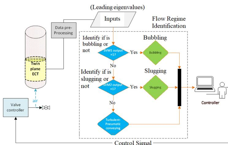
Figure 7. Flow chart of a FBC controller design scenario based on ECT sensor based on some machine-learning algorithms
