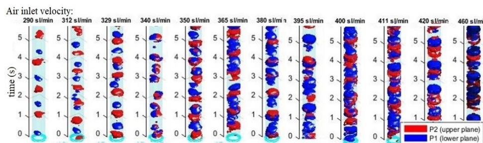
Figure 2. Reconstructed bubble images with airflow varying from 290 to 340SLM; 'blue' indicates the bubble generated from the lower ECT sensor plane (p1, relatively close to the bottom of bed and air inlet area); 'red' indicates the bubble generated from upper ECT sensor plane (p2).
