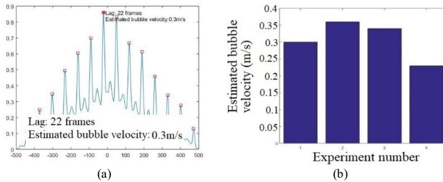
Figure 3. Cross-correlation based estimation of bubble velocity, 0.3 m/s, with air input flow rate at 292SLM; (b) estimated bubble frequency with the air inlet velocity from 290SLM to 340SLM
