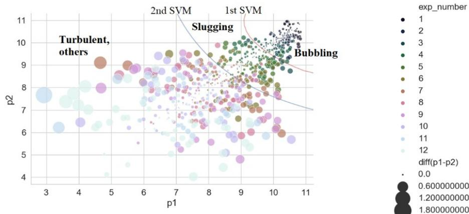
Figure 6. Overview of trained stacked SVM results; where 1<sup>st</sup> SVM (red hyperplane) is used to classify 'bubbling' and others; 2<sup>nd</sup> SVM (blue hyperplane) is used to classify between 'slugging' and 'turbulent, others'
