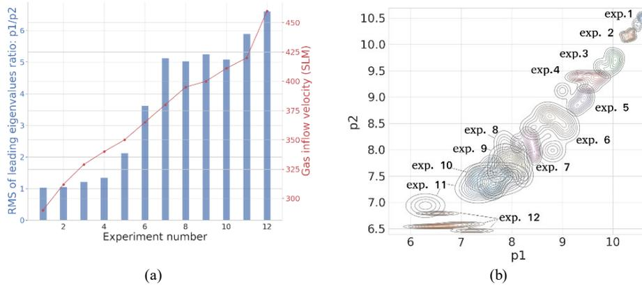
Figure 5. (a) RMS values of the ratios of leading eigenvalues for capacitance matrices measured at lower plane (P1) and upper plane (P2); the red dot and line plot is the corresponding air inflow velocity; (b) Kernel Density Estimate (KDE) plot: Data distribution of 10-second-averaged leading eigenvalues between P1 and P2
